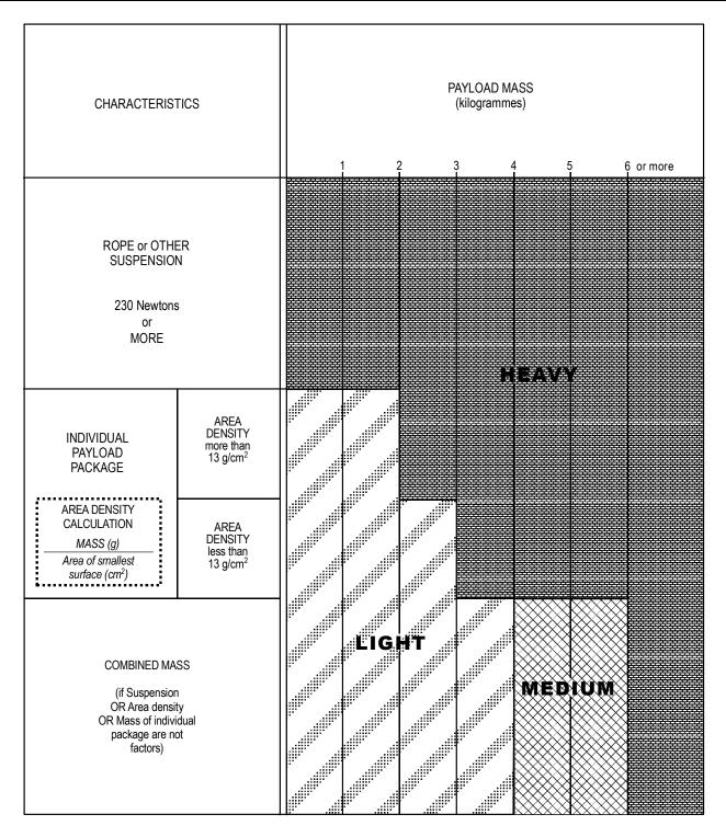
Figure A5-1. Classification of unmanned free balloons
