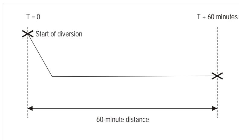
**Figure C-2. Sixty-minute distance — aeroplanes with two turbine engines**
