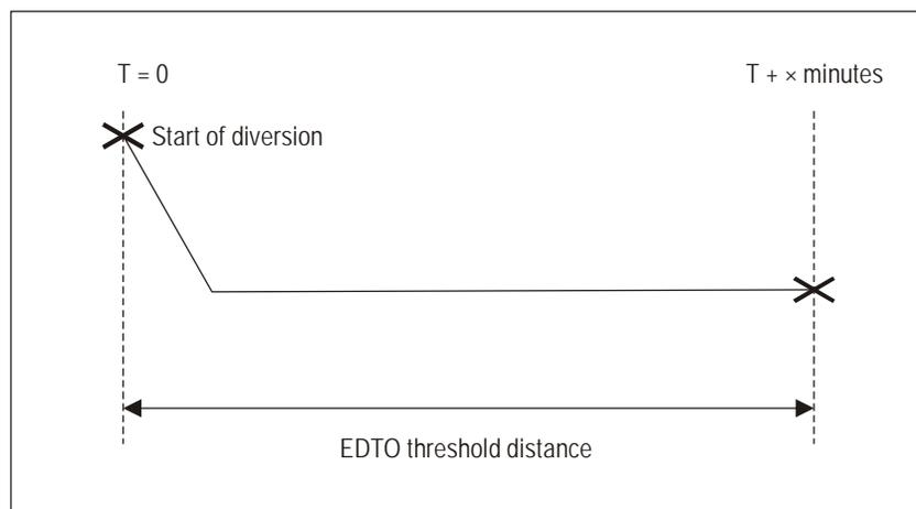
**Figure C-8. Threshold distance — aeroplanes with two turbine engines**
