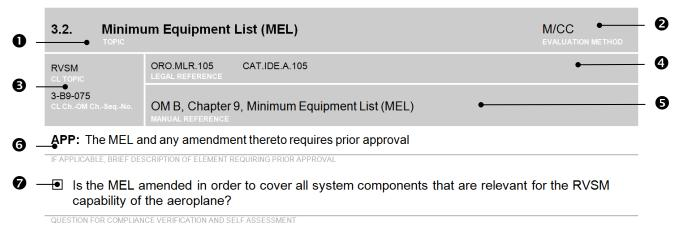
The MEL shall be amended in order to comply with the requirement for RVSM operations in respect to system capability and redundancy.
